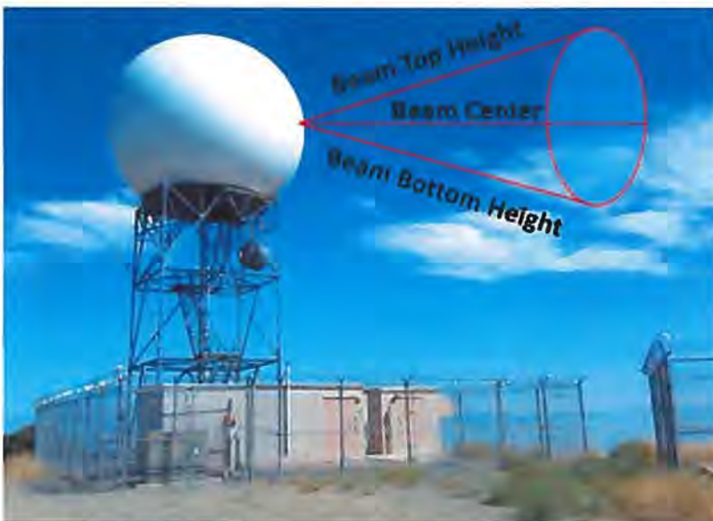
23 24 Figure 10. Illustration of the NEXRAD Radar Beam
